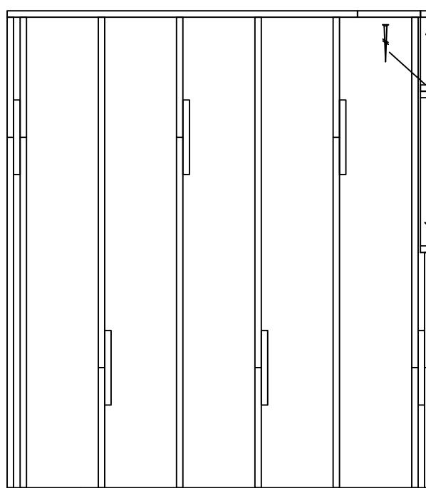
Fix wall element EL-1 with screws
