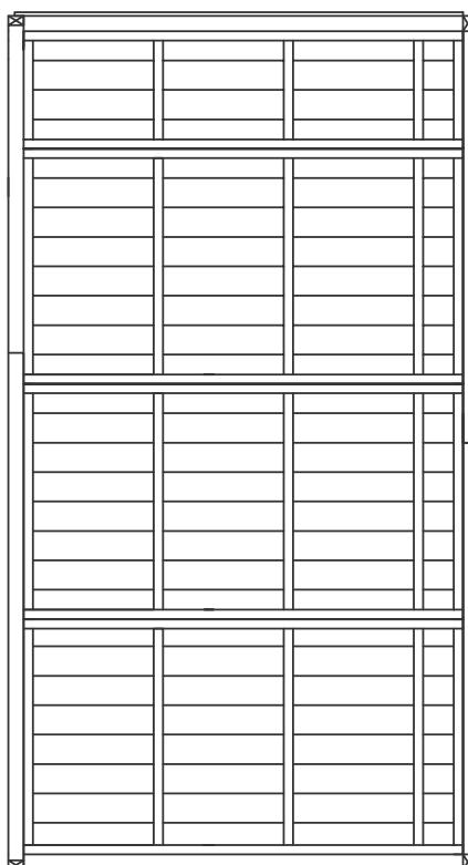
Fix wall element EL-5 with back wall elements with screws 5.0x120 together
