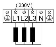
2.2 Connecting the heater to the power supply
