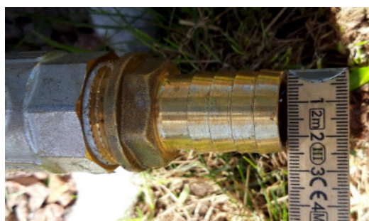
Dimension of the emptying tap 25 mm.
