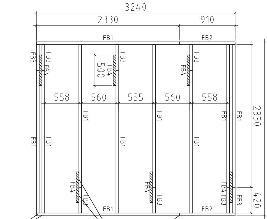
Connect with metal plate 60x160 +screws 4,5x45 2pc
