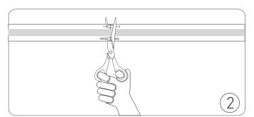
Measure the length of the surface, cut the COB strip need, please cut the COB strip according to the markings on the COB strip.
