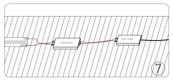
With Controller:connect the LED driver to the power supply secondly,then complete installation.
