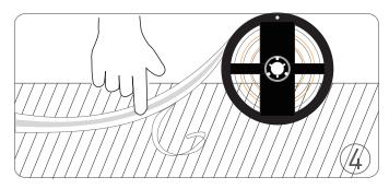
Tear the double sided adhesive tape and paste the COB strip to the surface, press the COB strip to stick to the surface tightly.
