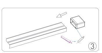
Use professional silicone adhesive, first squeeze into the needle, then the silicone tail plug inside coated with silicone adhesive, put into the lamp tail end, wait 3-5 hours, completely cured and can be installed
