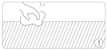
Clean the surface to make sure the surface free from grease, dust and liquid.
