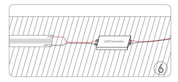
With controller:connect the COB strip to the LED controller firstly.
