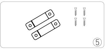
After installing COB strip light, install the mounting clip on the strip light, align the screws with the opening holes of the buckle, and tighten thescrews. It is recommended to use 2pcs per meter.
